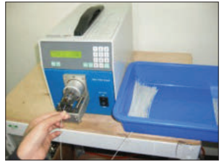
▲ Fig. 4 CMC semi-automatic stripper assures quality with precision and stable tolerance control.
